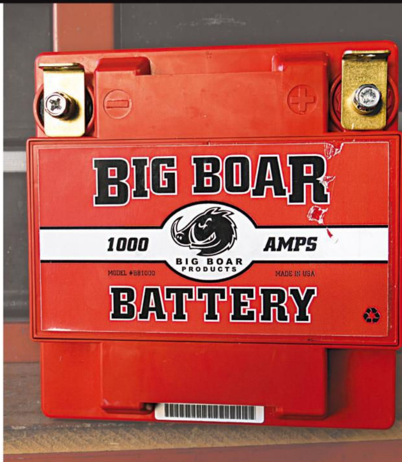
■ Our bright-orange 1,000-amp Big Boar battery ready to get installed in the '09 Road King.
