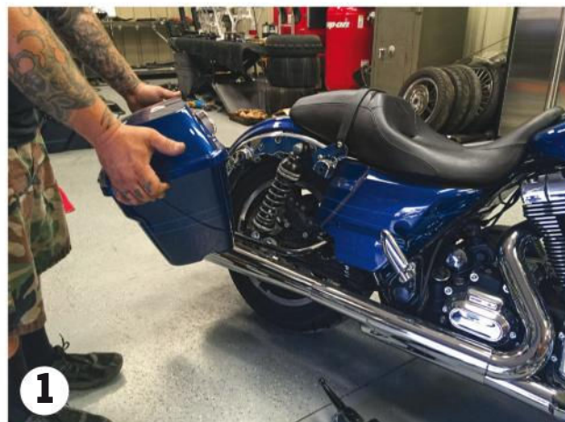
1 Josh started the installation by removing the right saddlebag in order to access the ABS module underneath the right side cover.
